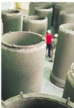
Concrete pipes at the new, highly automated Washington, Maryland, plant. CSR America has been constructing efficient low cost concrete pipe plants in new locations and replacing old plants.
